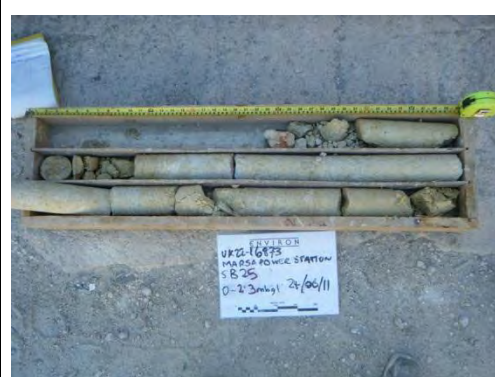
Photo 34. Rock core SB25 (0.0-3.0m bgl)
