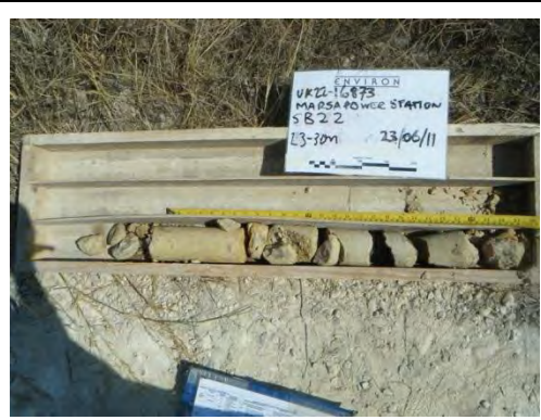
Photo 29. Rock core SB22 (2.3-3.0m bgl)
