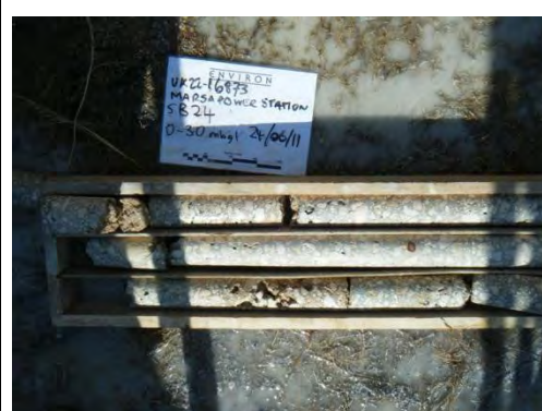
Photo 33. Rock core SB24 (0.0-3.0m bgl)
