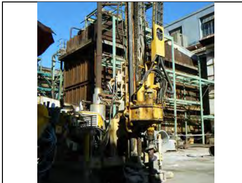
Photo 12. Beretta T44 drilling rig
