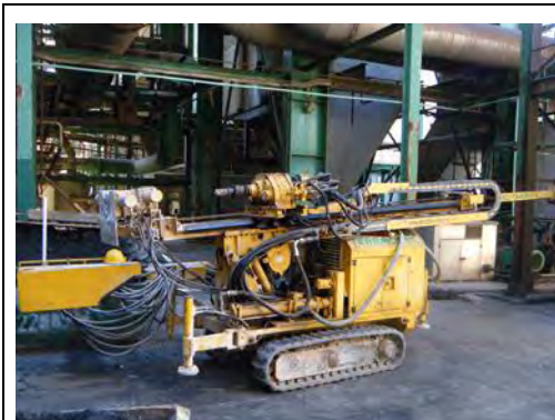
Photo 11. Beretta T44 drilling rig
