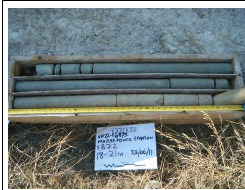
Photo 30. Rock core SB22 (18.0-21.0m bgl)
